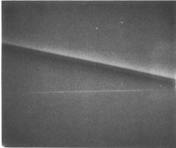
Figure 13 SEM of a smaller cleavage step where no secondary steps are evident. \times 3200 .
